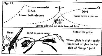
set the glue. Once this has cooled (usually 5 - 10 seconds) the joint will retain the new position. Adjusting in this fashion makes the addition of lead weight slivers unnecessary.
