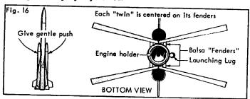
☐ 7. Slide the model down the launch rod (check for, and correct any binding tendency along the rod) make sure the safety key is out of the controller and connect the micro-clips to the igniter leads. (Remember -- clip 'em as close to the engine nozzle as possible.)
