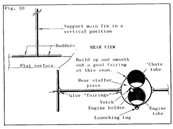
11. Glue one stuffer piece into place at the rear of the body tube on the side opposite the engine holder. Fit the remaining stuffer piece against its location and mark it on either side of the engine holder. Make a 1/8" notch (see fig. 10, rear view) to allow the engine holder to be sprung outward enough to release a spent engine casing. Glue the fitted stuffer piece in place taking care to get no glue on the engine holder.
